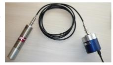
The device is therefore useful for obtaining the energy spectrum from the photon radiation detected by the scintillator, and can be easily interfaced to a typical PC or notebook via a standard USB port for further data transfer and analysis.
